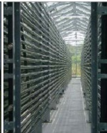
Fig. 3 A high-end closed bioreactor system. The worlds largest closed photo-bioreactor in Klötze, near Wolfsburg, Germany (Bioprodukte Prof. Steinberg; www.algomed.de ); the 700 m 3 are distributed in 500 km of tubes and produce up to 100 t algae biomass per year
