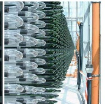
Fig. 3 A high-end closed bioreactor system. The worlds largest closed photo-bioreactor in Klötze, near Wolfsburg, Germany (Bioprodukte Prof. Steinberg; www.algomed.de ); the 700 m 3 are distributed in 500 km of tubes and produce up to 100 t algae biomass per year
